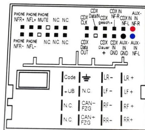
4. Now connect the black ground cable to the radio housing or the black line directly to a ground line to the radio connection (pin assignment GND symbol, next to the code). an. You can also use an alligator clip here. Without a good ground connection the function of the adapter is not given.
