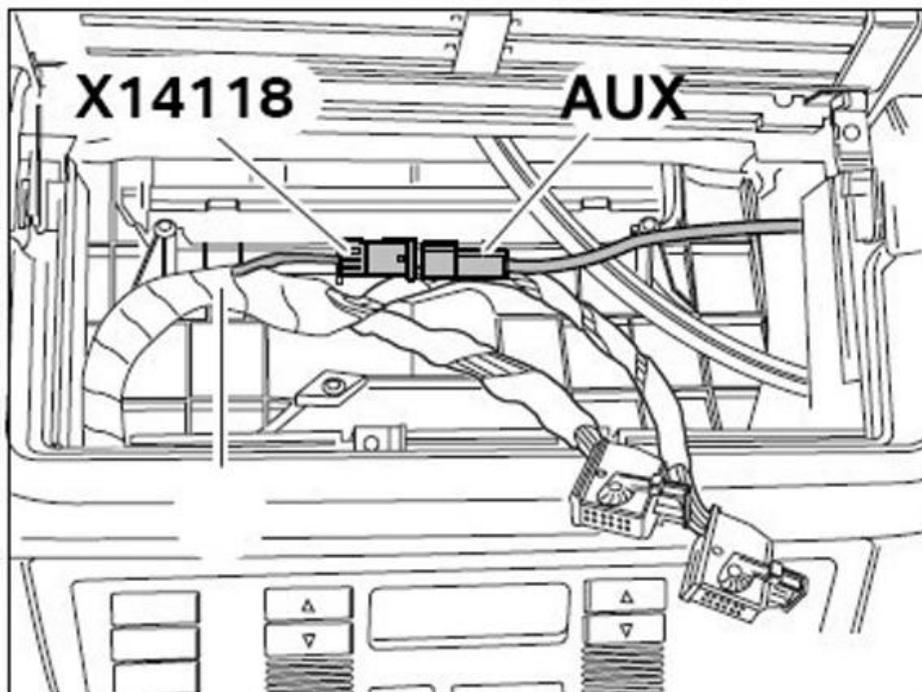
4. Now connect the black ground cable to the radio housing or the black cable directly to a ground cable to the radio connection (usually a thick brown cable). The function of the adapter is not possible without a good ground connection.
