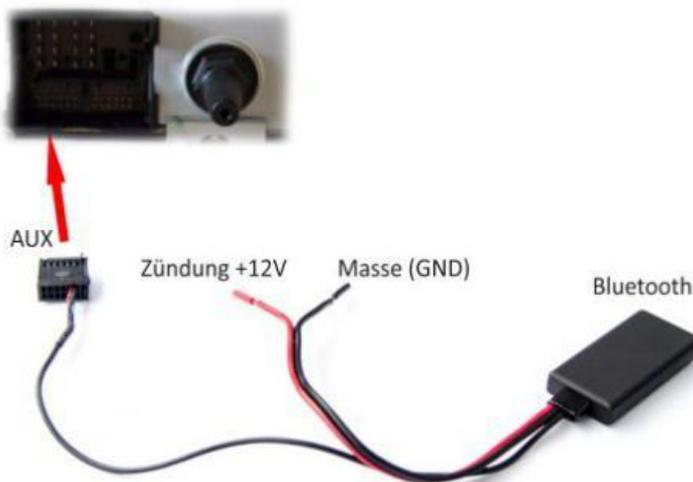
4. Now connect the black ground cable of the WM-BTMIC19 either to the radio housing or to the ground line leading to the radio. Without a good ground connection the function of the adapter is not given.
