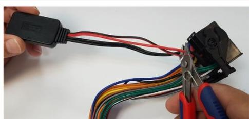
Cut the red cable that goes to the Bluetooth adapter directly behind the plug.
