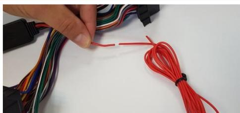
Now connect the red cable with the loose red cable, which is included in the scope of delivery.
