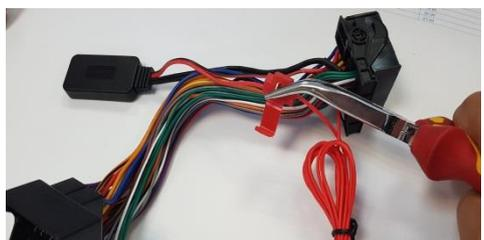
Use one of the cable thieves supplied for this purpose. Then press in the metal pin with a pair of needle-nose pliers.
